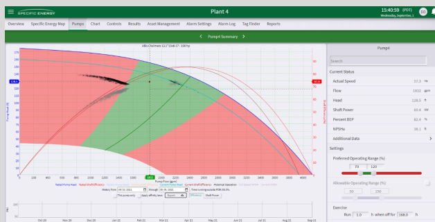
A real-time plot of Pump Head vs. Pump Flow for a single pump, which allows the City of Lakewood to evaluate the operating efficiency of the pump and make adjustments as necessary.
